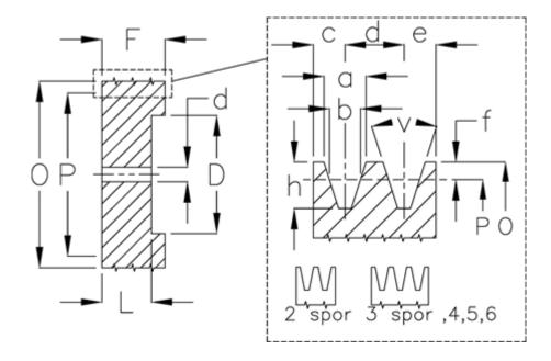
$\begin{array}{lll} D & = 67 \\ d & = 15 \\ F & = 80.0 \\ L & = 52 \\ Number of ribs = 5 \\ O & = 105.5 \\ P & = 100 \\ Type & = A \end{array}$
